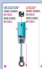
Extend the shock shaft completely. Fill the shock body with the shock oil. For the FRONT shocks use 700cSt or 600cSt oil. For the REAR shocks use 550cSt or 500cSt oil.
