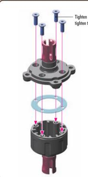
Tighten the screws equally but DO NOT tighten them completely.
