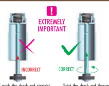
DO NOT push the shock rod straight Twist the shock rod through through the lower shock body assembly; O-ring damage may result.
